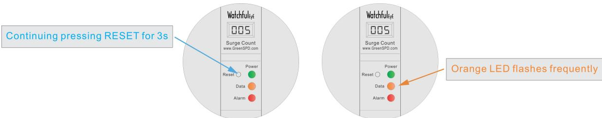
2. When Modbus indicator flashes frequently, short press RESET to set RS485 ID address (RS485 ID: 1-247)
